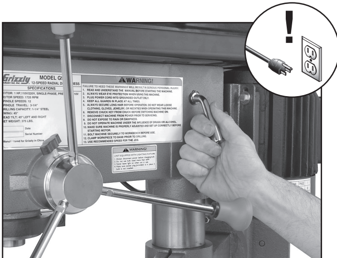
Figure 21. Using the belt tension lever.
